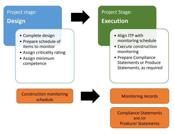
Figure 1; Key Elements of Risk-based Construction Monitoring Framework
